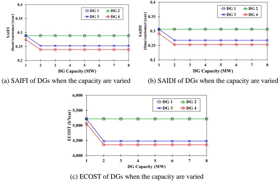
Fig. 2. The reliability indices of system connected to DGs
