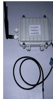
Fig. 5. Temperature sensor node placed in spot.
