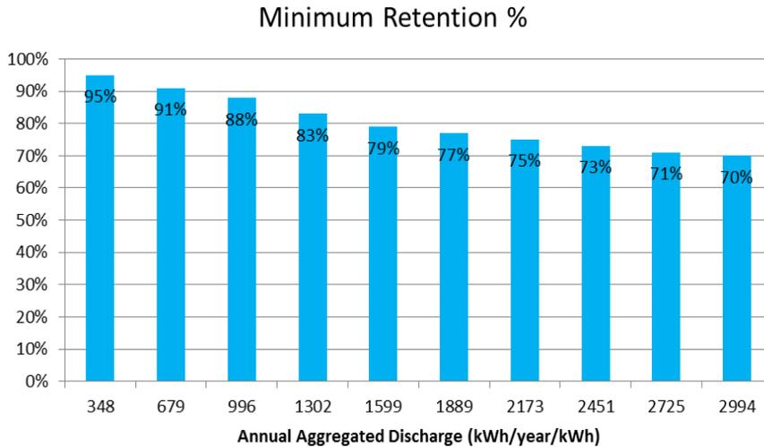
Fig. 6. Battery model annual retention regime as a function of cumulative annual discharged power
