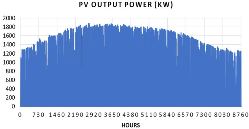
Fig. 5. PV capacity output power profile
