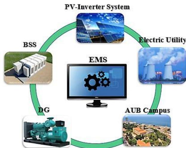
Fig. 1. Proposed system configuration
