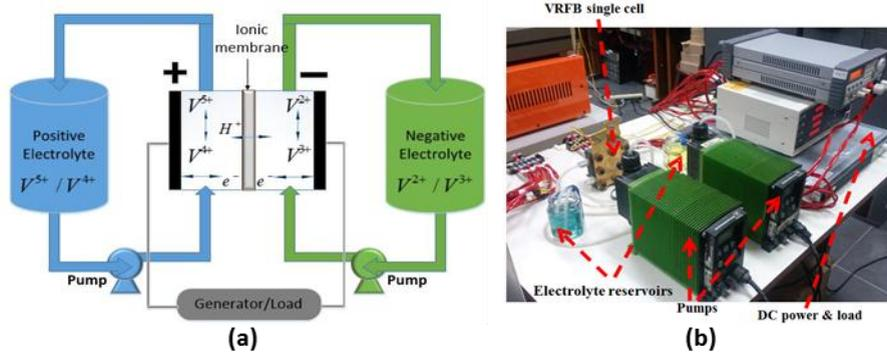
Fig. 1. (a) VRFB operation principle, (b) VRFB single cell experimental system.
