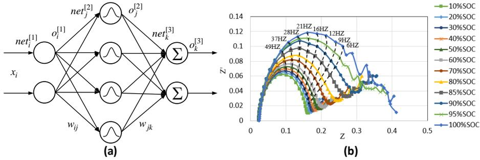
Fig. 2. (a) BPNN architecture, (b) EIS data obtained from the VRFB cell system in Fig. 1 (b).
