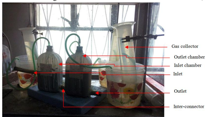
Fig. 3. Experimental setup of the daily feed double chamber reactor.
