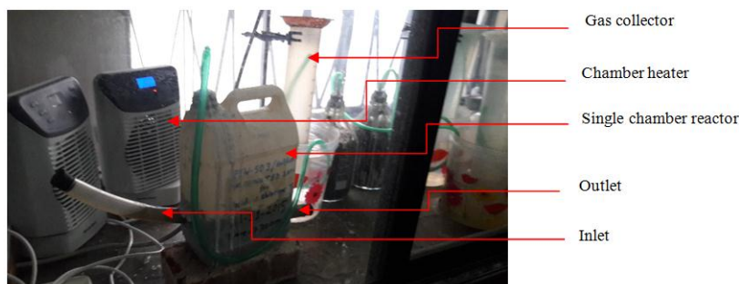
Fig. 2. Experimental setup of the daily feed single chamber reactor.
