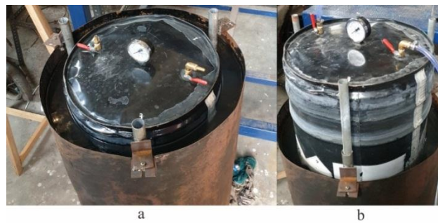
Fig. 7. Hydrogen gas storage tubes (a) the tubes sink empty; (b) the tube floats when filled with gas.
