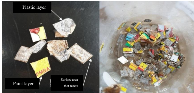
Fig. 9. Samples of used aluminum beverage cans that is not completely reacting
