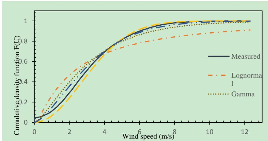
Fig. 2. Cumulative distribution functions compared with the measured curve.
