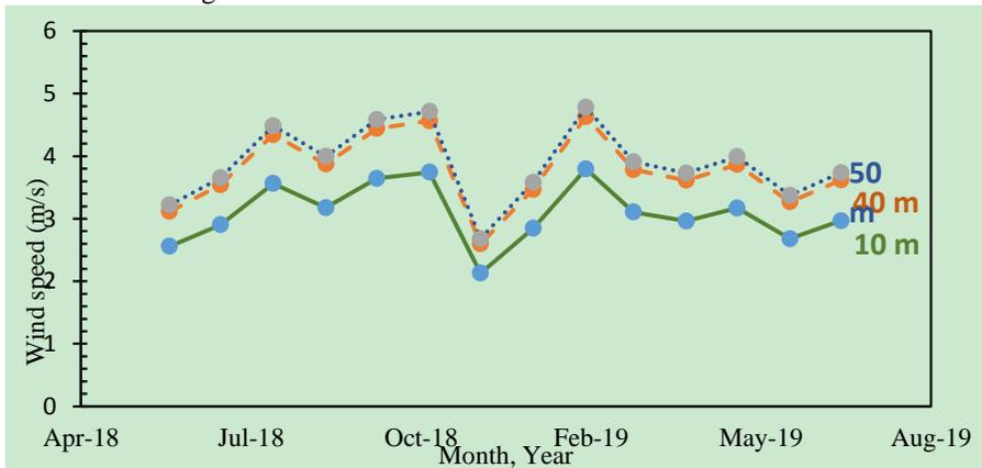
Fig. 6. Monthly average wind speeds for the following heights: 10m, 40m, and 50m.
