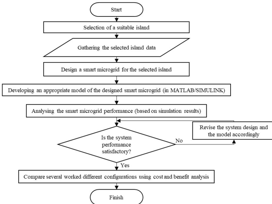
Fig. 1. Smart Microgrid Design and Analysis Workflow
