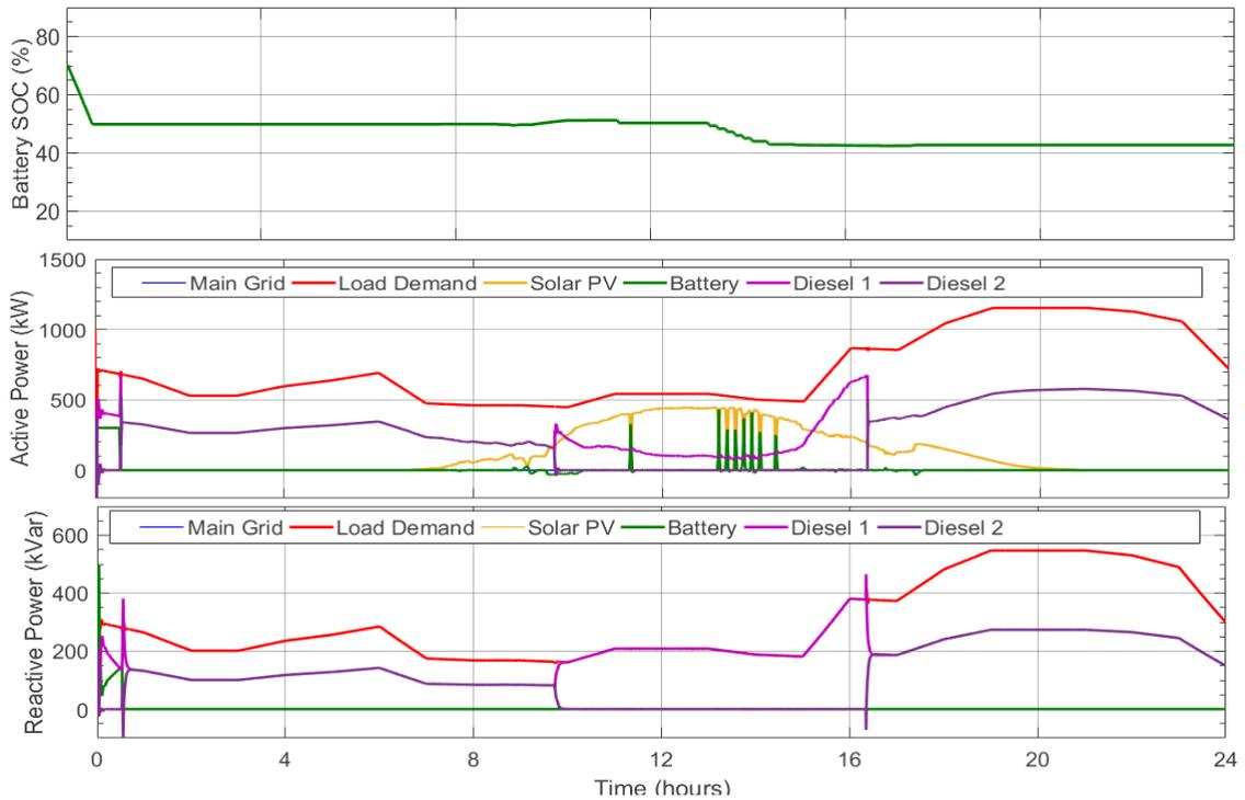
Fig. 4. Microgrid performance simulation results in the islanded mode scenario
