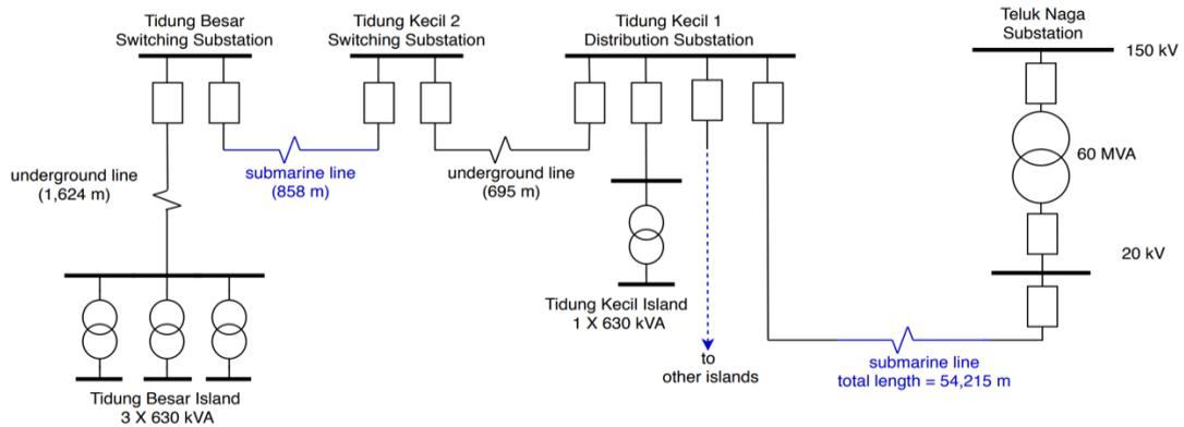
Fig. 2. Simplified single line diagram of Tidung island (adapted from [18])
