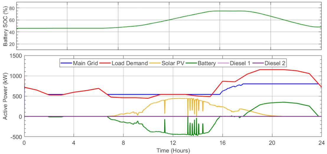
Fig. 6. Simulation result of peak shaving using ESS with 7,400 kWh battery
