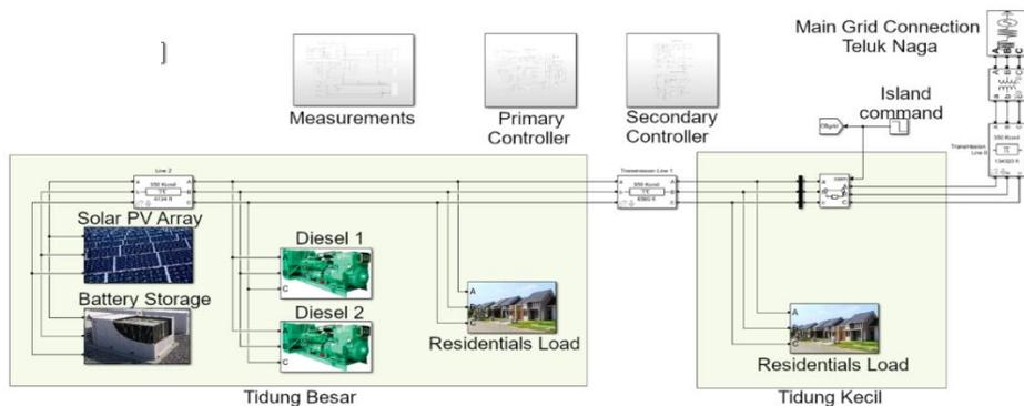
Fig. 3. Simulink model of Tidung island smart microgrid
