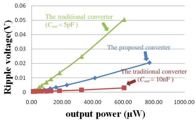
Fig. 7. Simulated ripple voltage as a function of the output power.
