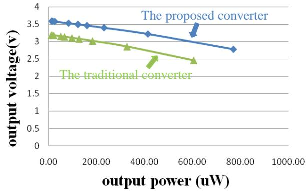
Fig. 6. Simulated output voltage as a function of the output power.
