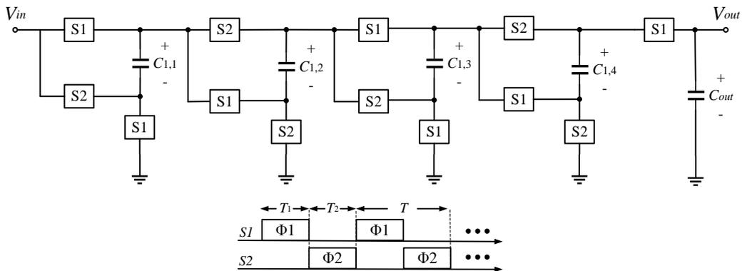
Fig. 1. Circuit configuration of the 4-stages traditional Fibonacci converter.
