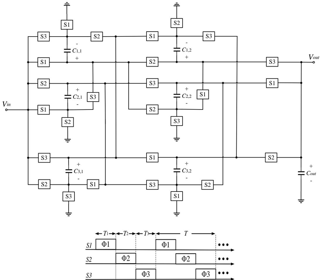
Fig. 2. Circuit configuration of the 2-stages proposed converter.
