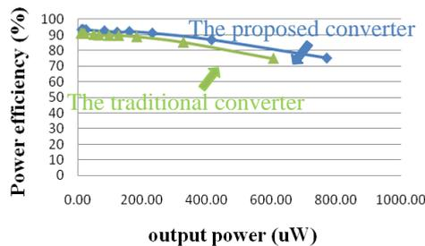
Fig. 5. Simulated power efficiency as a function of the output power.
