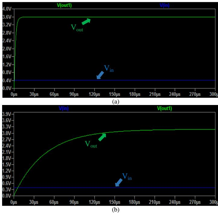
Fig. 8. Simulated output voltage as a function of time: (a) proposed converter and (b) Fibonacci converter.
