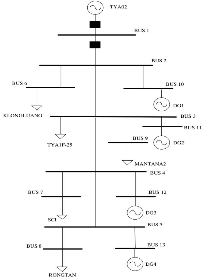
Fig. 1 The single-line diagram of the distribution system of the Thanyaburi substation
