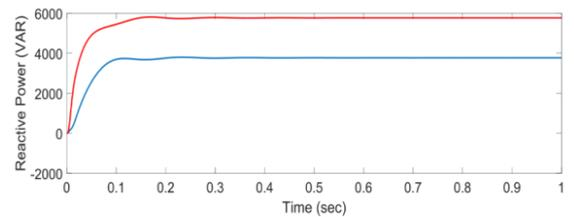
Fig. 5. Reactive Power: Conventional PI Controller
