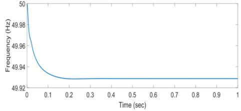
Fig. 11. Frequency: Proposed Controller
