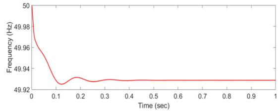
Fig. 7. Frequency: Conventional PI Controller
