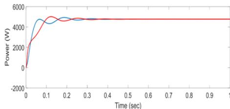
Fig. 4. Active Power: Conventional PI Controller
