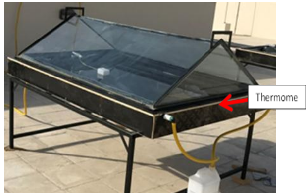
Fig. 2. Photograph of the double-slope solar still
