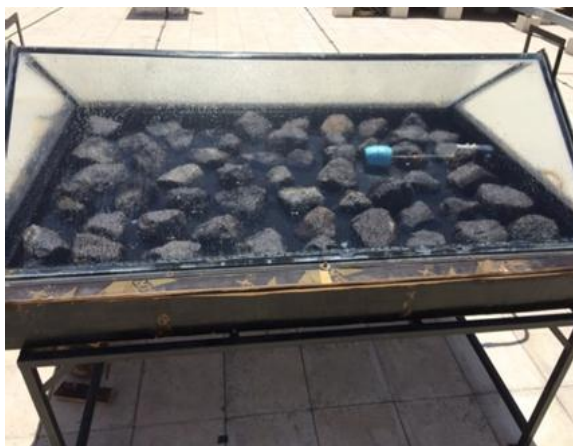
Fig. 4. Double-slope solar still with igneous rocks.
