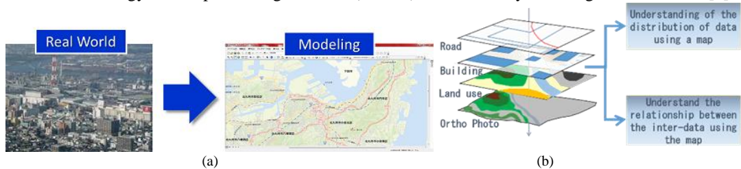
Fig. 1. GIS utilization: (a) GIS image and (b) GIS principle.
