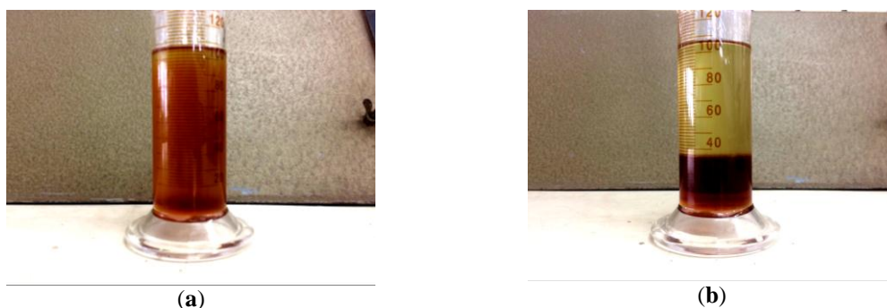
Fig. 5. Biodiesel from palm oil process: (a) Before e-field supply (b) After e-field supply.
