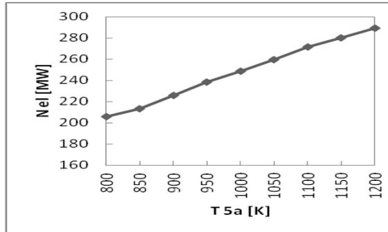
Fig. 6. Impact of supplementary firing on Net power of 1P.
