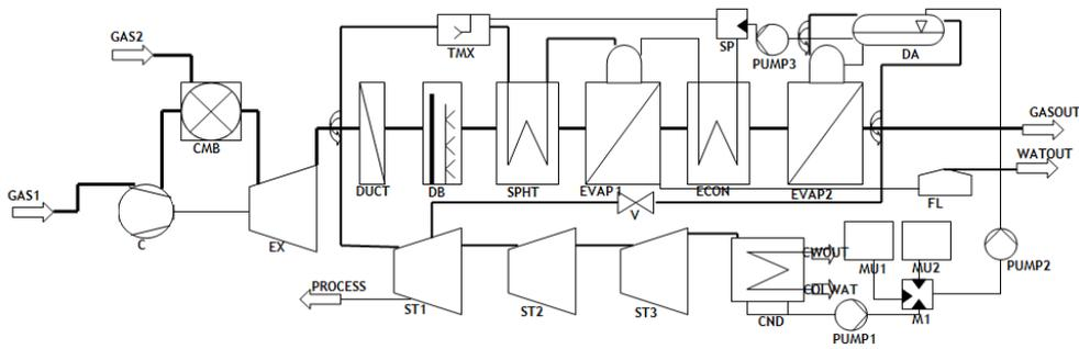
Fig. 2. Dual-Pressure combined cycle power plant.
