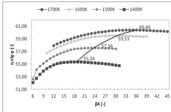
Fig. 8. Relation between electric power efficiency, pressure ratio and gas turbine inlet temperature of 3PR.
