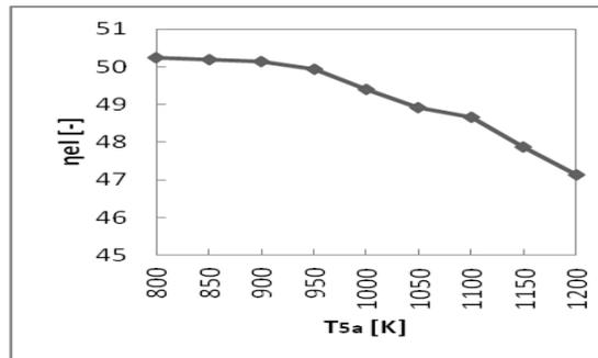
Fig. 5. Impact of supplementary firing on electric power efficiency of 1P.
