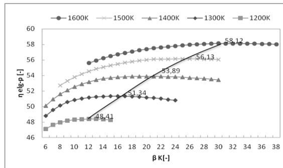
Fig. 7. Relation between electric power efficiency, pressure ratio and gas turbine inlet temperature of 2P.
