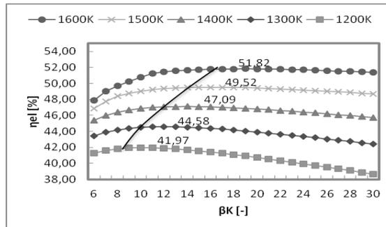
Fig. 4. Relation between electric power efficiency, pressure ratio and gas turbine inlet temperature of 1P.
