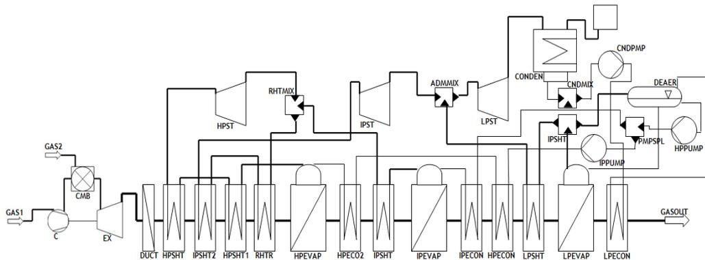
Fig. 3. Triple-Pressure reheat combined cycle power plant.
