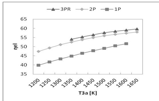
Fig. 9. Comparison of impacts of temperature on the inlet to gas turbine on three different cycles: 1P, 2P, 3.
