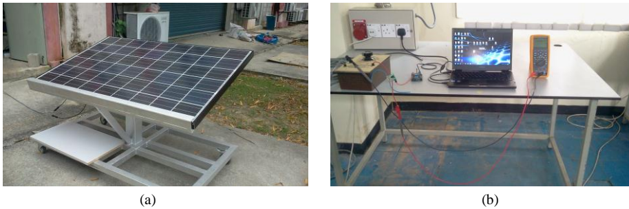
Fig. 6. Set up for the test bed of ZigBee1Sensor integrated with Arduino at remote location for measuring PV current (a) PV panel (b) ZigBee1 is connected with PV panel to retrieve PV generated current (1.5 A).
