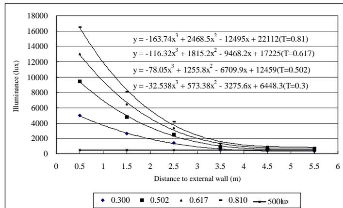
Fig. 1. Variation of indoor illuminance with glazing transmittance in sunny day
