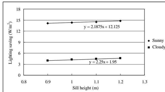
Fig. 6. Variation of lighting saving with sill height
