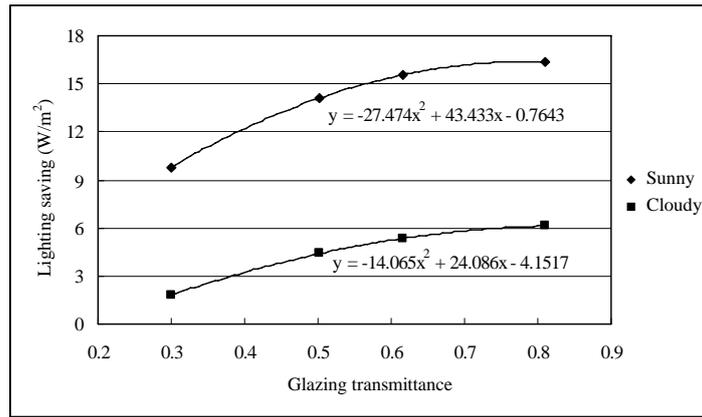
Fig. 3. Variation of lighting saving with glazing transmittance
