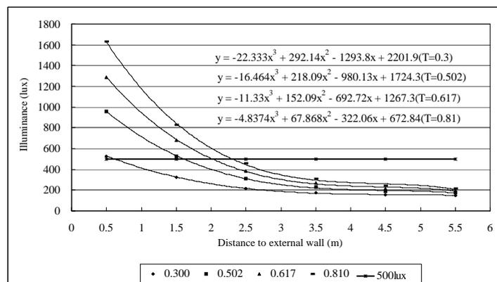
Fig. 2. Variation of indoor illuminance with glazing transmittance in cloudy day
