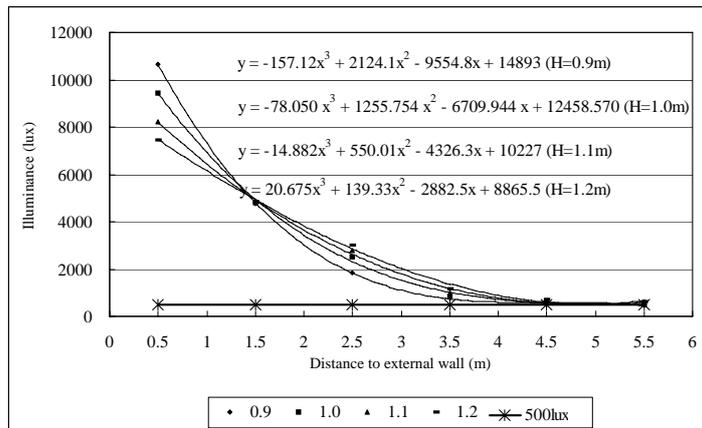
Fig. 4. Variation of indoor illuminance with sill height in sunny day
