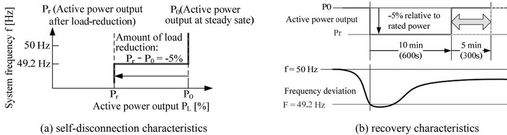
Fig. 1. Proposed self-disconnection characteristics and recovery characteristics of residential air-conditioner.
