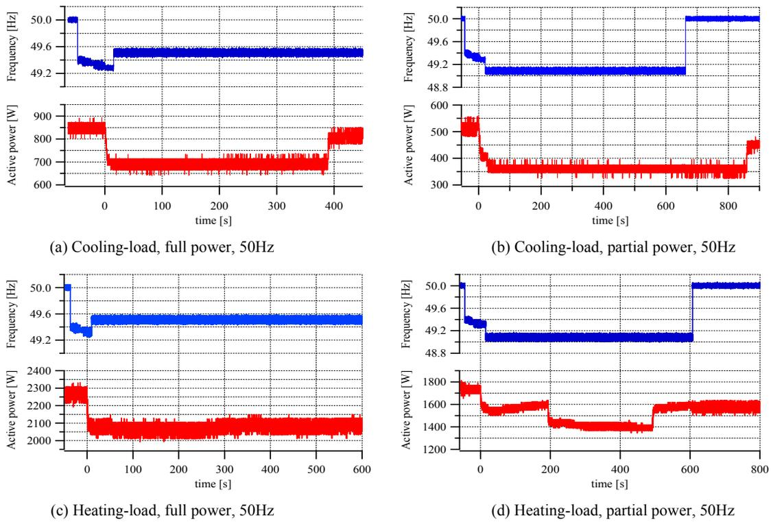
Fig. 4. Measured response of frequency and active power consumption of AC.
