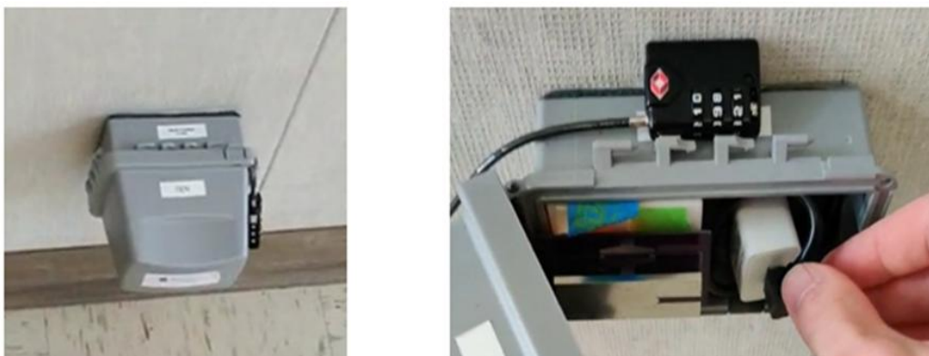
Fig. 5. TruePODS plugged in to AC outlet. Protective enclosure (left), and microSD card access (right).
